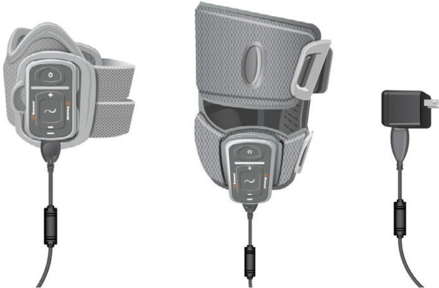
Figure 6-2: L300 Go System Charging Setup (Example of a Lower Leg FS Cuff and Thigh Cuff Configuration)
